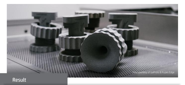
With the assistance of HP DMN partner GoProto, Ropes Edge used HP Multi Jet Fusion technology to perfect their design and produce faster and less expensively than what was possible with traditional manufacturing methods.
